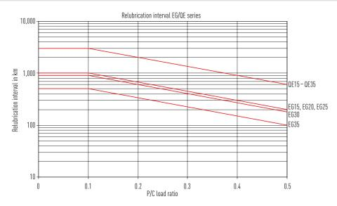
Fig. 6.27 Load-dependent relubrication intervals for grease lubrication - EG series
