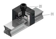
Fig. 4.12 Pressing in of the bolt cap by tightening the screw (2)
