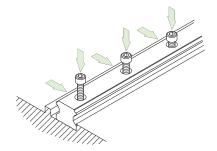
Fig. 4.5 Adjusting the rail on the bed and assembly of the screws
