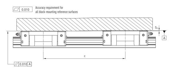
Fig. 4.21 Maximum height tolerance  $S_3$
