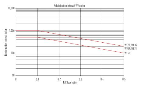
Fig. 6.28 Load-dependent relubrication intervals for grease lubrication – WE series
