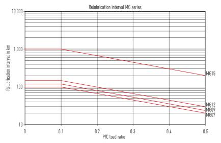
Fig. 6.29 Load-dependent relubrication intervals for grease lubrication – MG series
