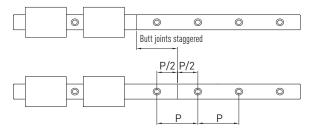
Fig. 4.30 Configuration of jointed multi-part rails
