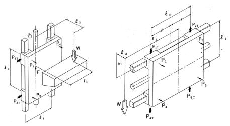
Fig. 6.18 Mounting positions of profile rails
