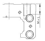
Fig. 4.27 Depiction of bore hole and recirculation channel
