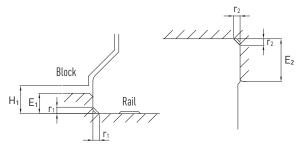
Fig. 4.26 Shoulder heights and fillets – RG/QR series
