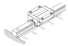
Fig. 4.6 Tightening the push screws
