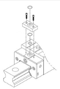
Fig. 6.17 Structure of the lubrication adapter
