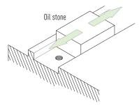
Fig. 4.3 Cleaning the mounting surface
