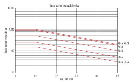
Fig. 6.31 Load-dependent relubrication intervals for grease lubrication – RG series
