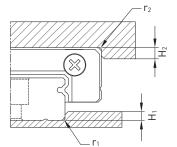
Fig. 4.25 Shoulder heights and fillets - MG and PM series
