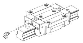
Fig. 6.1 Lubrication connection on the front side
