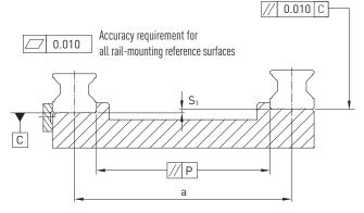
Fig. 4.19 Parallelism of the reference surface P - RG/QR series
