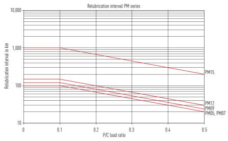
Fig. 6.30 Load-dependent relubrication intervals for grease lubrication - PM series
