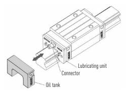
Lubrication passes from the oil cartridge via the connector to the lubricator which then lubricates the track of the rail. Due to the specific design of the oil tank, the block can be assembled in any position without influencing the lubrication effect. The replacement intervals of the oil tank depend heavily on the loads and the environmental conditions. Environmental influences such as high loads, vibrations and dirt shorten the replacement intervals.
