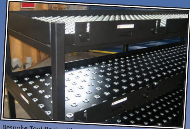
Bespoke Tool-Rack with sunk Ball Transfer Units
