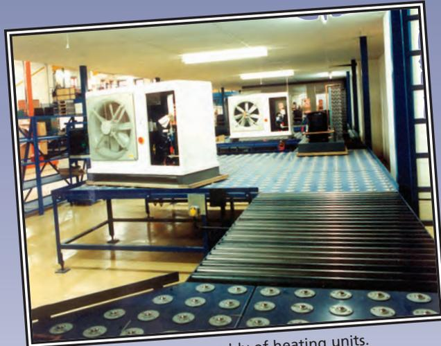
Ball units used for the assembly of heating units.
