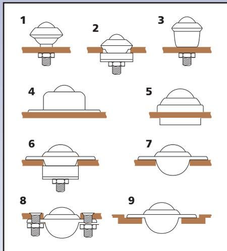
There are various methods of fixing Alwaysse ball units. A wide range of fittings enable them to be used with various different materials.
