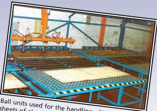
Ball units used for the handling of large sheets of aluminium.
