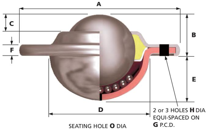
Ball unit Ref. No's 1022 and 1035 with solid steel inner ring (SI) option illustrated with no seal for improved protection from shock loading.
