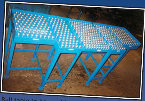
Ball table to be used in an assembly area.
